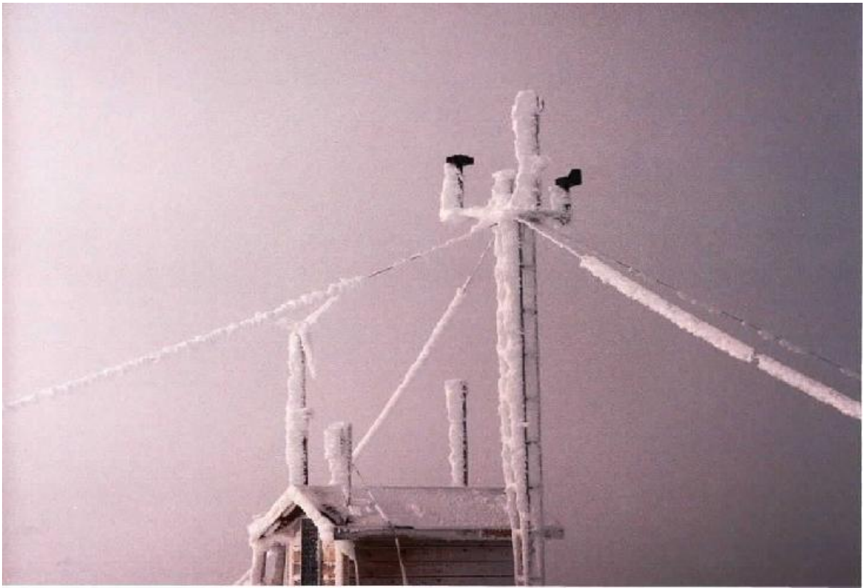
Photograph 1: Rime ice on monitoring equipment, only heated instruments stay clear
