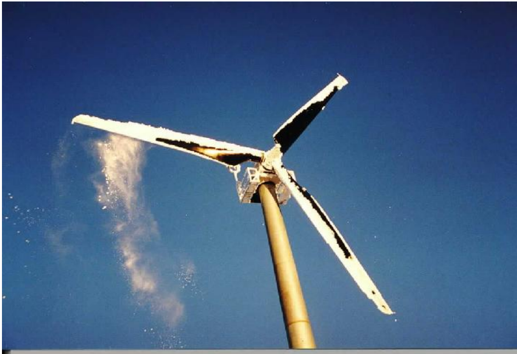
Photograph 8: accumulated ice shedding from black blades
