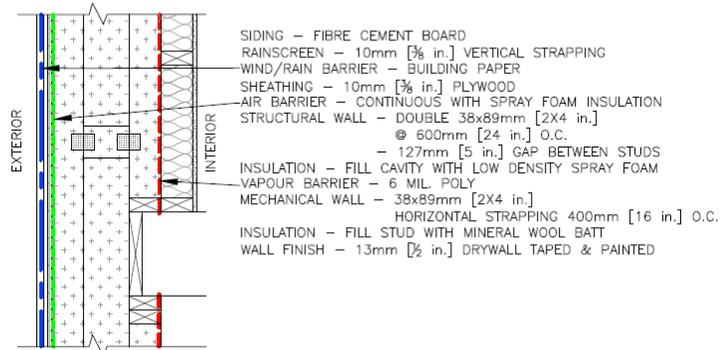
Figure 2: Wall section
