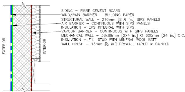
Figure 4: Wall section
