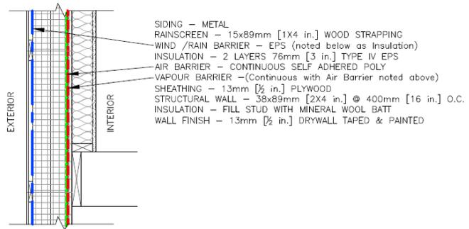
Figure 2: Wall section
